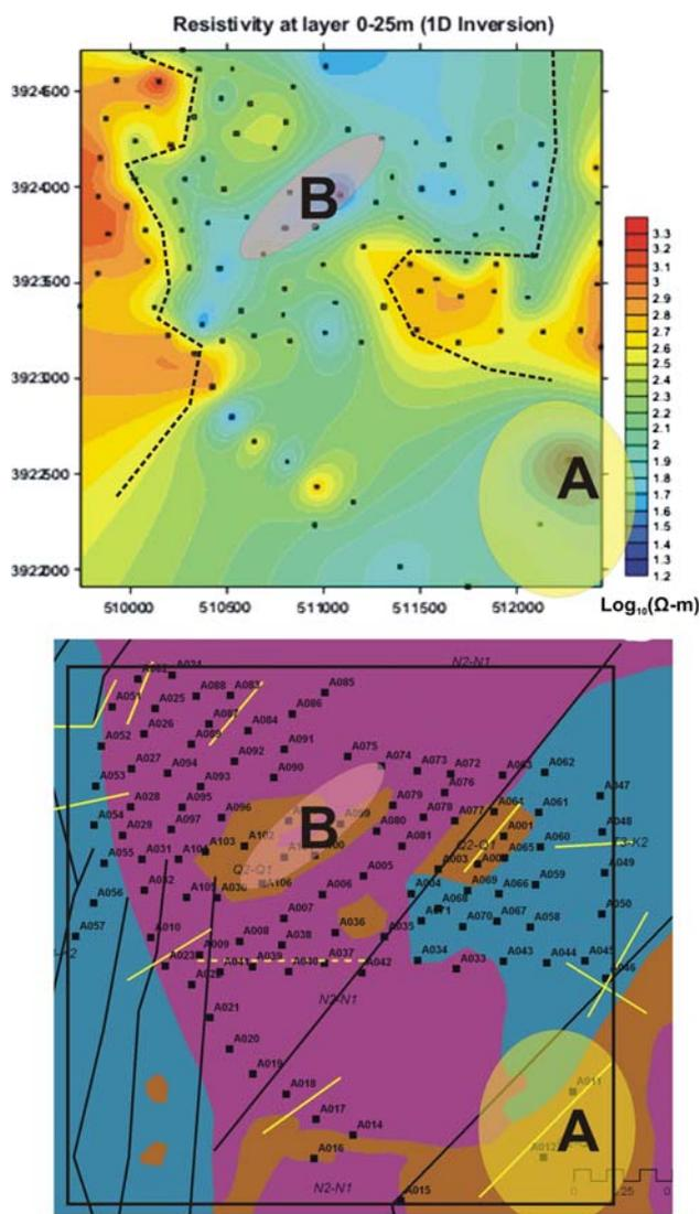
**Fig. 8** Comparison between the shallower geophysical slice and the regional geologic field map is presented. Two low-resistivity areas are found (A and B), which correlate with saltwater intrusion and shallow aquifer, respectively. Based on the shape of the contact between the geophysical units, two fault zones are assumed and verified by the geological mapping
