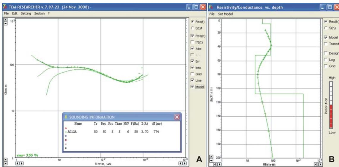
**Fig. 5 a** Curve of apparent resistivity  $\rho_a(t)$  (example of sounding A012A). Two more curves are given as a result of the raw data smoothing. The first (upper) continuous curve approximates initial  $\rho_a(t)$  data and the second (lower) curve is the calculated dependence
