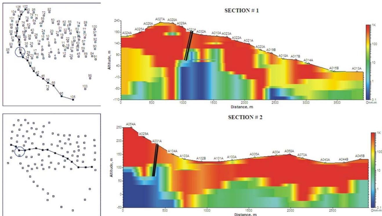
**Fig. 6** Two-dimensional representation of the resistivity distribution in depth are given for a NW–SE and W–E profiles. The suggested location for the construction of a hydrowell is presented by the *double black lines* at sounding A031A
